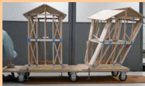
Experiment on the Simplified Version “Wooden House Collapse Bu-Ru-Ru”
